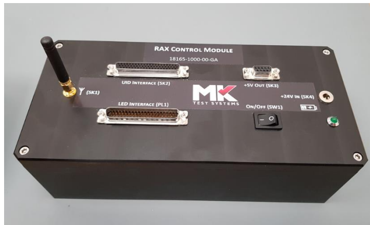
Control module fitted inside each trolley
